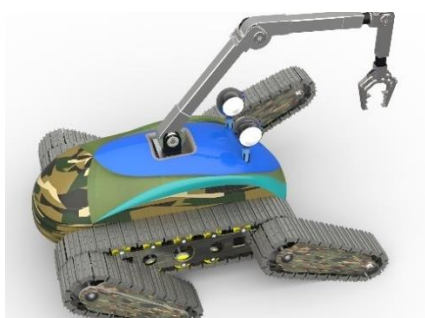
Fig. 1. The rescue robot with six tracks
