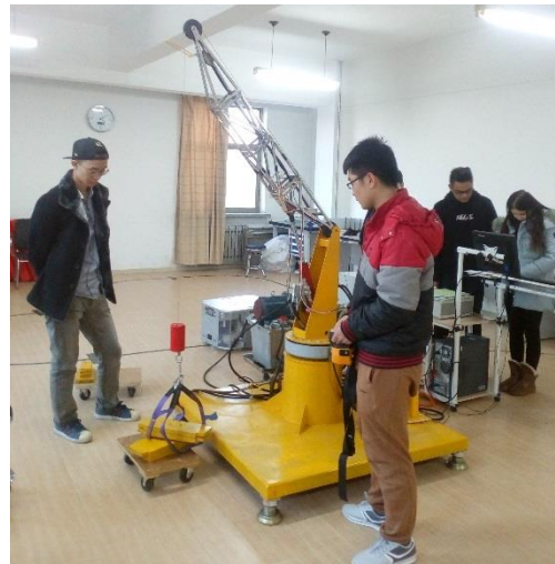
Fig. 2. Juniors are measuring boom dynamic stress
