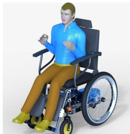
Fig. 3. The voice-controlled wheelchair
